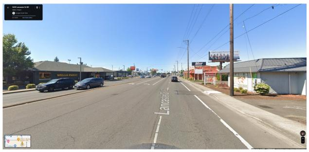
In this image, we can see the extent of the car-centric infrastructure on Lancaster Drive NE. We see a roadway with 6 wide lanes. The sidewalk, while present, is scattered between entrances into various shopping or otherwise commercial complexes We see a lack of trees and natural shading. It is obvious that when this layout was constructed, pedestrian comfort was an afterthought.
