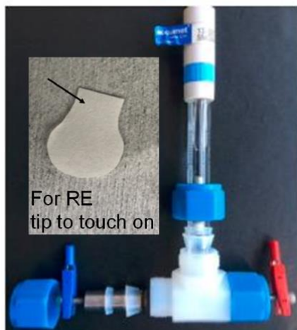
Figure A.8 Three-electrode custom Swagelok cells
