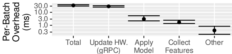
(b) Characterization of the batch-round-robin update time overhead with 100 prefixes per batch.
