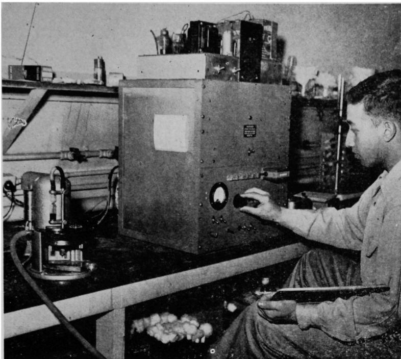
After removing a mammary gland and adding radioactive material, the scientists put the mixture into this device, a special kind of Geiger counter. The measurements help reveal how milk is produced.
