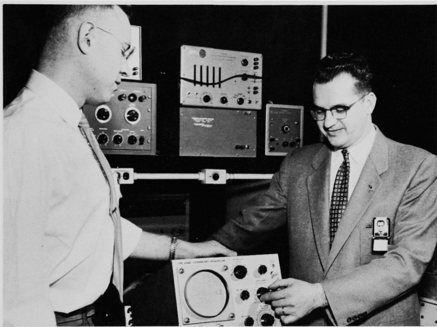
Dr. R. S. Paul (right), manager of testing methods, engineer section at Hanford, adjusts dial of a cathode-ray oscilloscope, an instrument used to analyze electrical wave forms. In photo below, Dr. Constantine H. Spalaris studies properties of reactor materials. He has since transferred to another General Electric plant in California.
