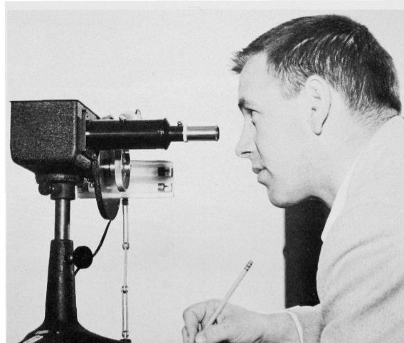
Byron B. Brenden, who works in the instrument research and development operation, uses a spectograph to check characteristic wave lengths of different light sources.
