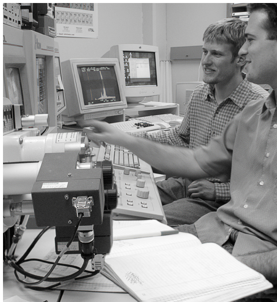
Electron beam lithography: UO researchers Nick Liebrecht (foreground) and Kurt Langworthy etch a 20-nanometer pattern on silicon to make nanoelectronic devices using equipment in the UO's MicroAnalytical Facility.
