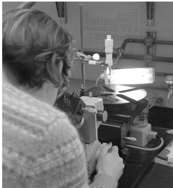
Contact angle goniometry: Using a device donated by Intel Corporation, UO chemistry Ph.D. student Jenny Dahl employs a classic technique for looking at nanoscale films on surfaces.
