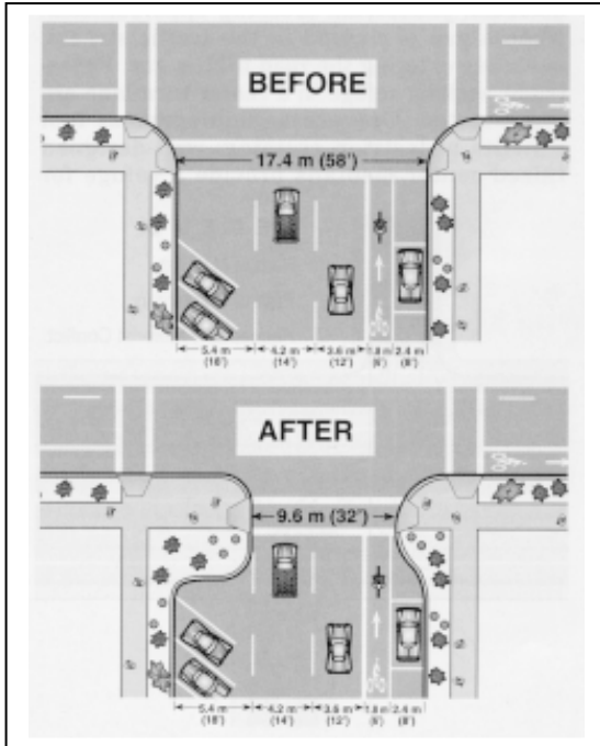
Figure 21. Example of curb extension Retrofit
