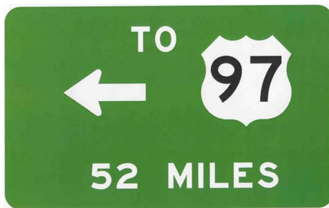
Figure 6-8. Example of Route Designation Sign and Directional Arrow Sign
