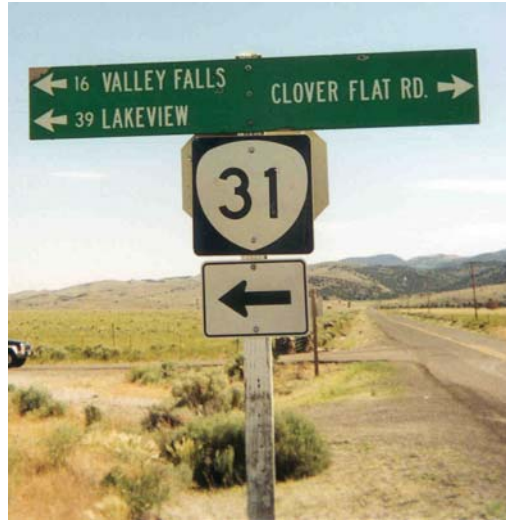
Figure 6-9. Example of Directional Signing identifying Distance and Direction to Specific Locations
