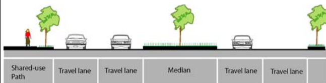
The existing roadway with an 8-10-foot-wide path along the outside of French Prairie Drive.
