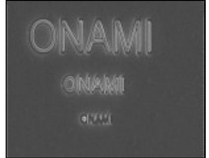
**Electron beam lithography is used to etch patterns into surfaces. Shown here at 9000x magnification during the news conference announcing the NSF instrumentation grant is the word "ONAMI," "written" with a beam of electrons into a piece of silicon.**
