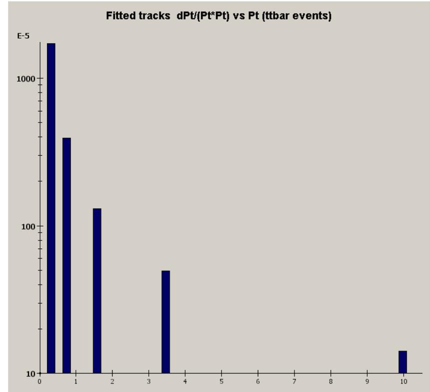
$P_t$  error  $dP_t/(P_t^*P_t)$  vs  $P_t$  for fitted tracks in  $t\bar{t}$  events (vertical scale in units of  $10^{-5}$  tracker resolution in  $R\phi$  is assumed  $7 \mu$ )
