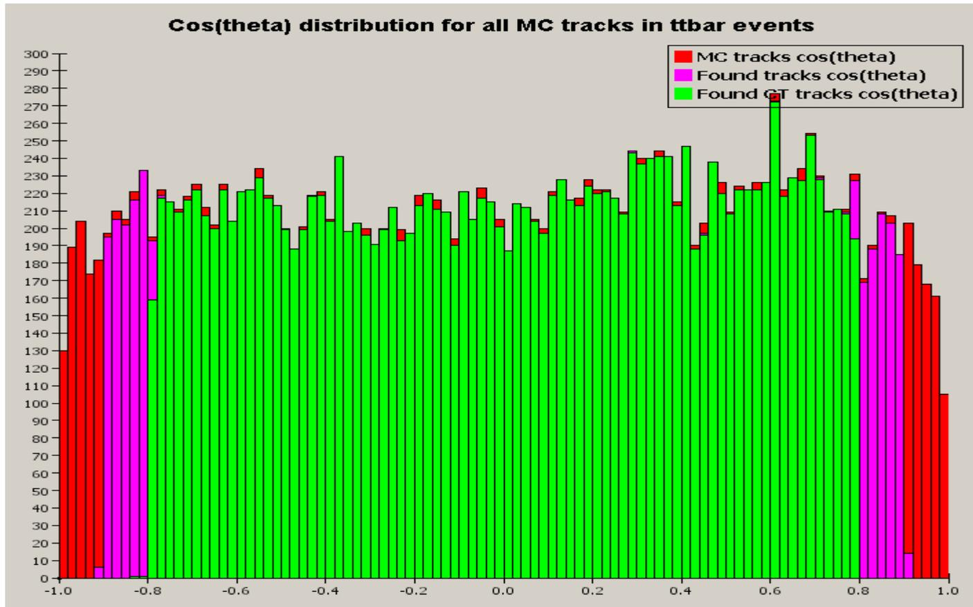
Cos( $\theta$ ) distribution of all tracks seen in tracker both central and endcap for ttbar events and for reconstructed tracks. Green histogram is reconstructed tracks with all hits seen in central tracker (this is only where current version of fitter can fit tracks with tracker hits included )
