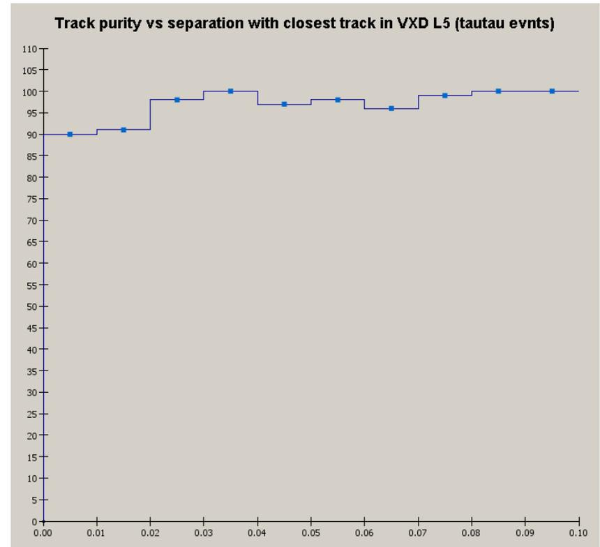
Purity of reconstructed tracks (fraction of hits having same MC parent) vs separation in LR5 of VXD (tautau events)
