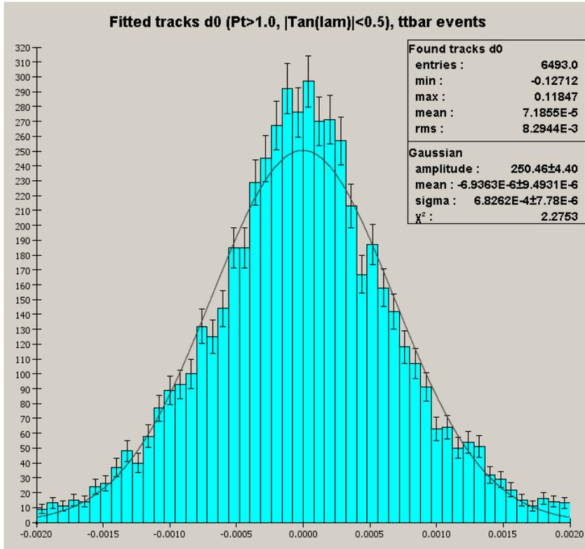
Impact parameter  $d_0$  distribution for fitted tracks ( $P_t > 1$  GeV,  $\tan(\lambda) < 0.5$ ) in  $t\bar{t}$  events.  $\sigma = 6.8 \mu$
