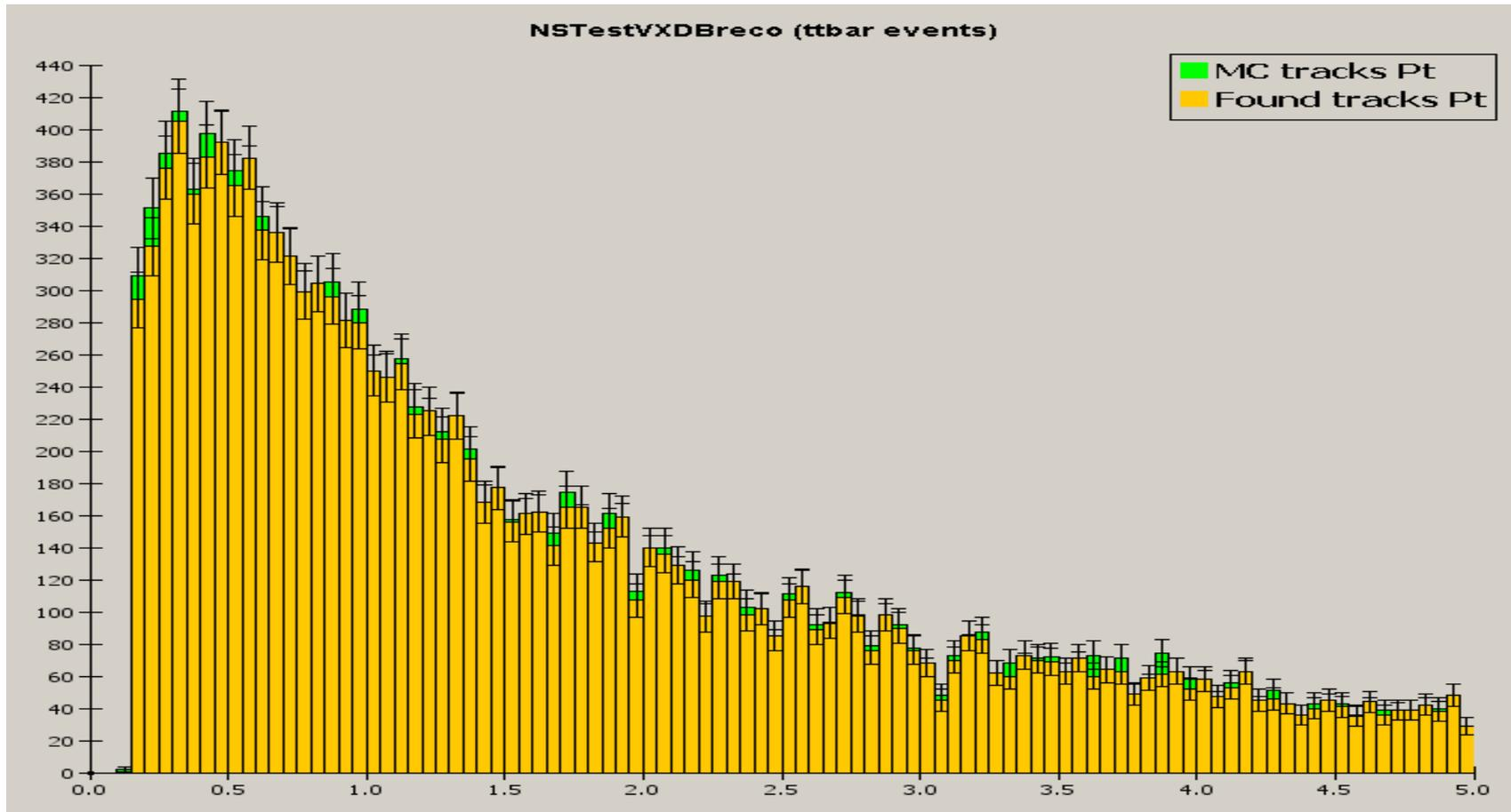
Pt distribution of Monte Carlo truth tracks in ttbar events for tracks within Reconstruction fiducial volume and of reconstructed tracks
