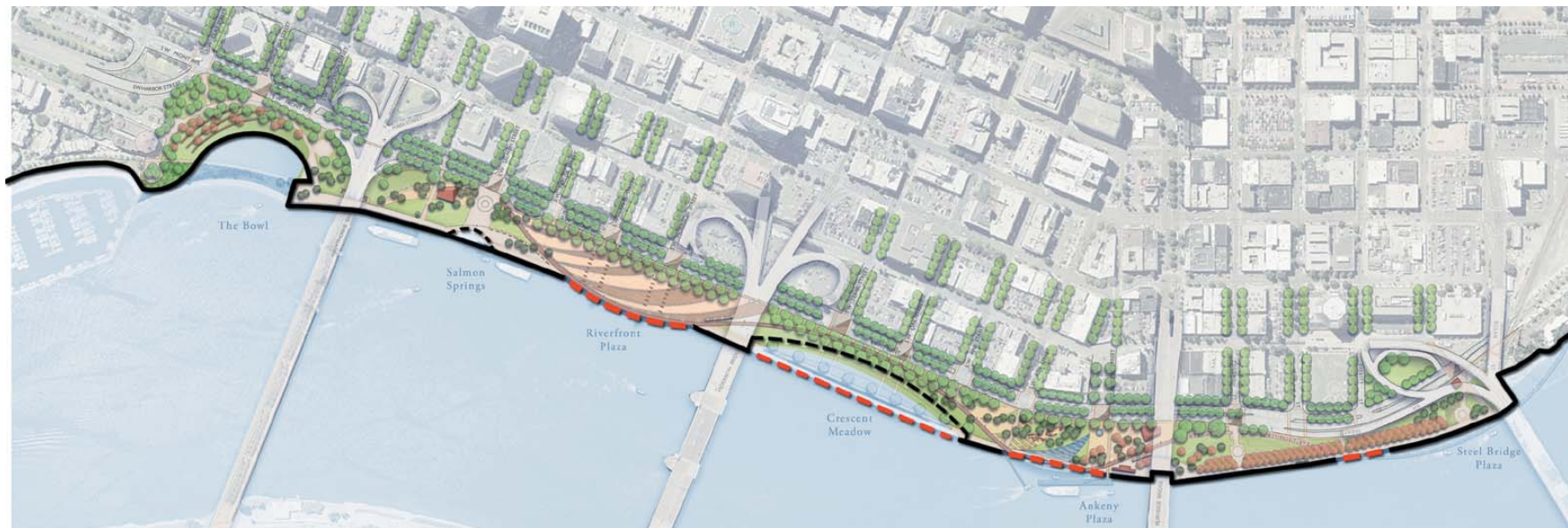
Diagram showing alterations to the seawall proposed by the Master Plan (in red), and the extent of flooding during the 100 year flood.
