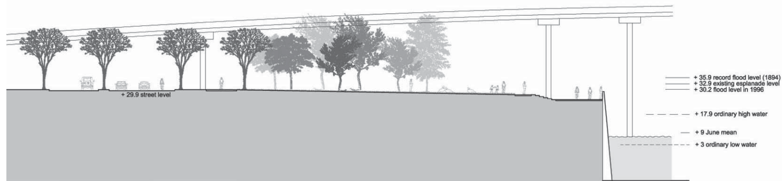
Section through the Meadow, looking north.
