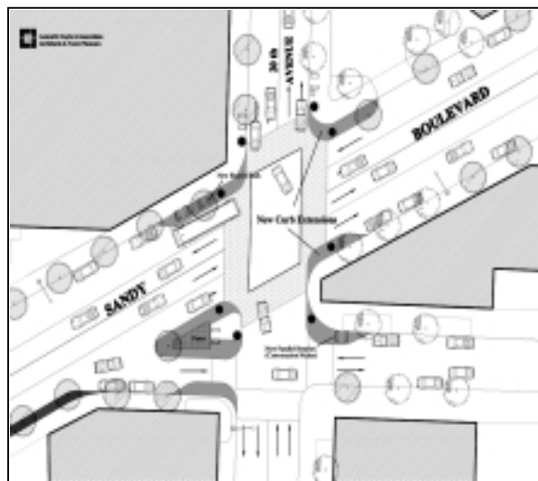
Redesigned intersection at NE 20 th Avenue and Sandy provides pedestrian amenities
