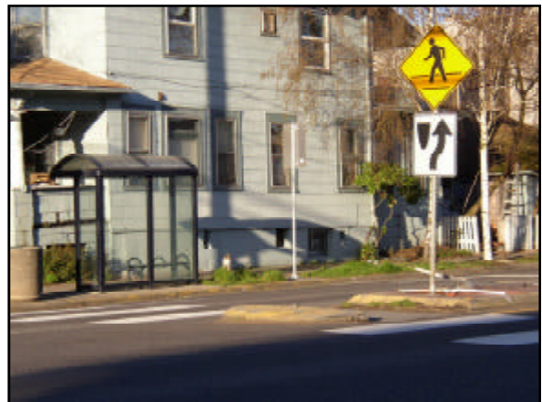
A pedestrian refuge island at East Burnside Street and 24th Avenue.
