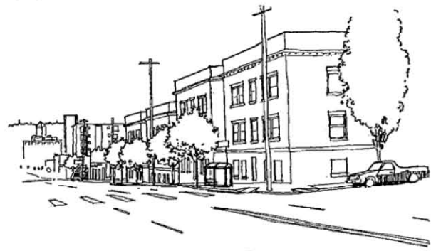
Curb extensions at transit stops provide extra room for shelters and amenities, and allow buses to stop in the travel lane, thereby decreasing the delay for transit.
