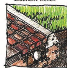
(c) Rumble strip with sediment trench
