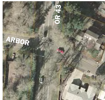
The OR 43/Arbor intersection is currently experiencing difficulties; existing ROW may allow for left turn lanes onto Arbor, but volumes do not warrant a signal to help traffic turning onto OR 43
