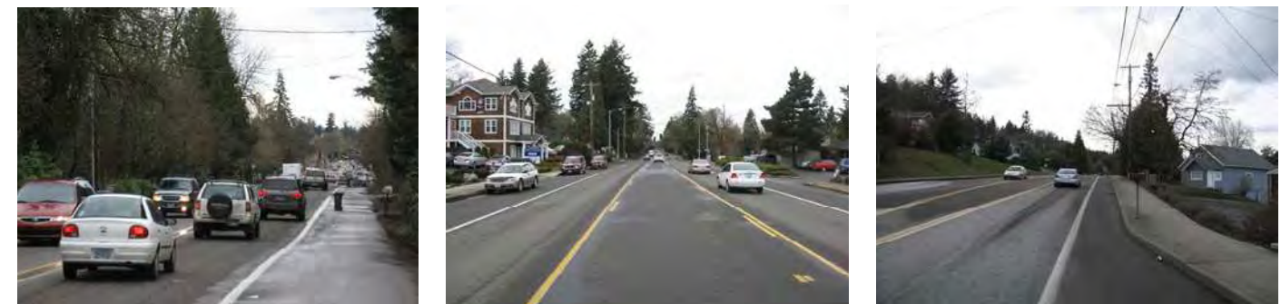
Examples of existing cross sections along OR 43 - based on available width, adjacent land uses, and transportation demands
