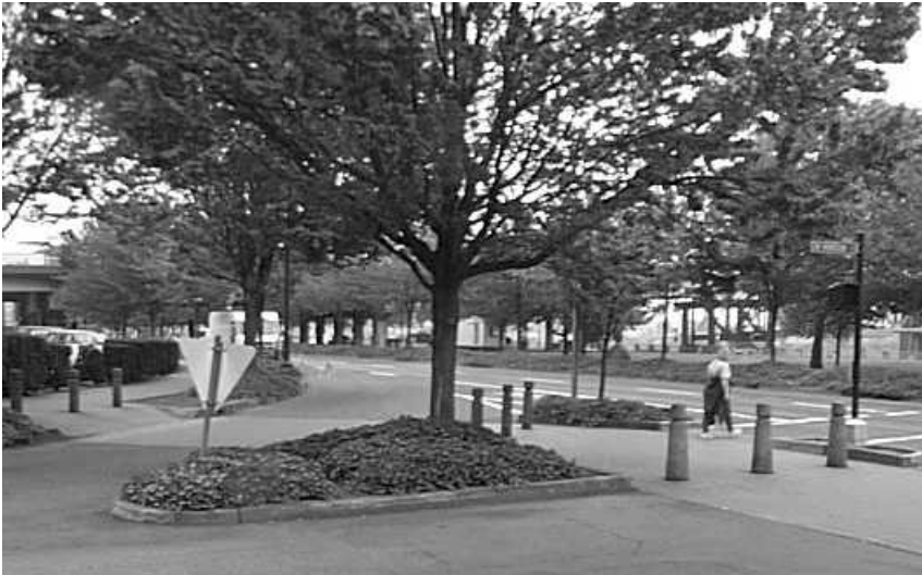
Refuge island on SW Front Street
