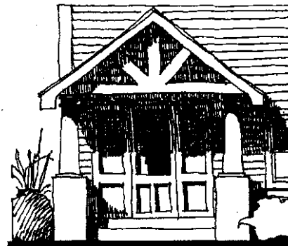
Porches with exposed rafters & interesting columns break down apparent size
