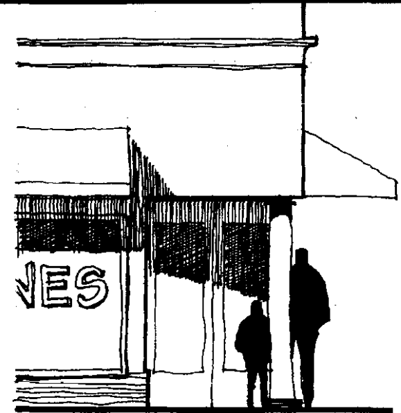
Corner Entry: Provide accessibility to both streets of the intersection and create a sheltering entry.
