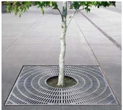
Manufacturer: Ironsmith, Inc http://ironsmith.cc/ Model: Starburst, 4814-1 Material: Cast iron; meets standards for class 35B gray iron per ASTM A48. Expandable; available in square, half round/half square and rectangular.
