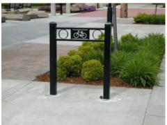
Manufacturer: CycleSafe Website: http://www.cyclesafe.com/VintageRacks.tab.aspx Model: Cascade Material: Schedule 40 steel pipe with 12-20 mil Armortec Plastisol coating. Available with bolt down or cast-in mounting. Cast-in mounting recommended.
