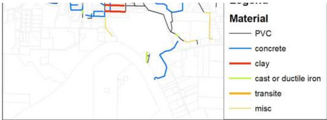
Figure D-3. Pipe material distribution in the Newberg collection system
