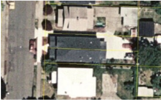
This paired rowhouse project, with only 50 feet of street frontage, illustrates that rear parking can be achieved on even very small sites. Note, however, that this results in most of the backyard being paved. The designer of these rowhouses indicated that it was somewhat more expensive to do rear parking, but that it did not significantly impact the affordability of the project.
