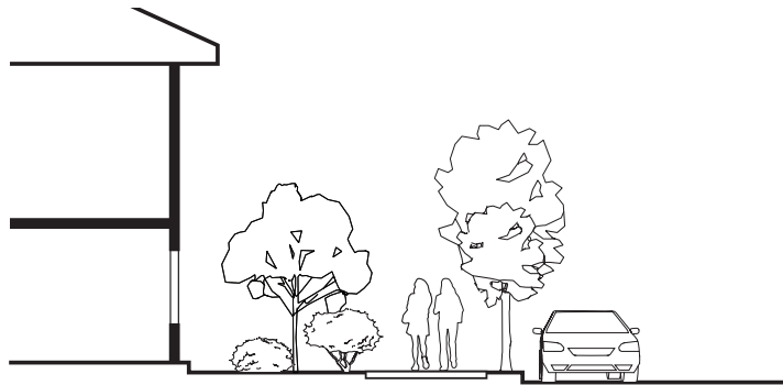
Ground-level units in this apartment building are both buffered from the street by a landscaped setback and raised above sidewalk level
