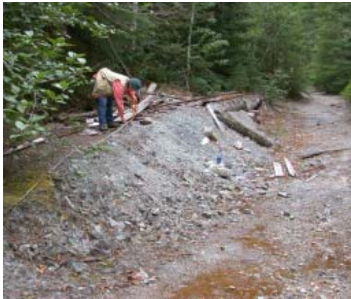
Photo 2. Level 5: Ore Car Track and Possible Loading Site. Niton Sample ID 28. Lead 4810 mg/kg. (photo by D. Boles)
