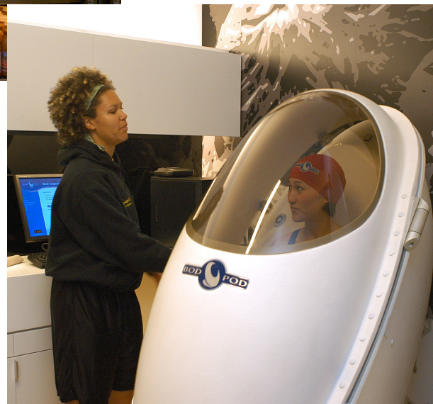
James Harris' assistant, GTF dietician Jessica Wilson, gets ready to take body fat measurements with the Bod Pod. This futuristic-looking machine determines lean body mass by measuring air displacement and density. Subjects must wear spandex body suits and hair coverings to ensure accurate readings.
