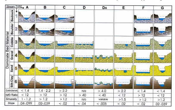
Figure 1. Delineative Criteria and Characteristics for the Major Stream Types (Rosgen 1996).
