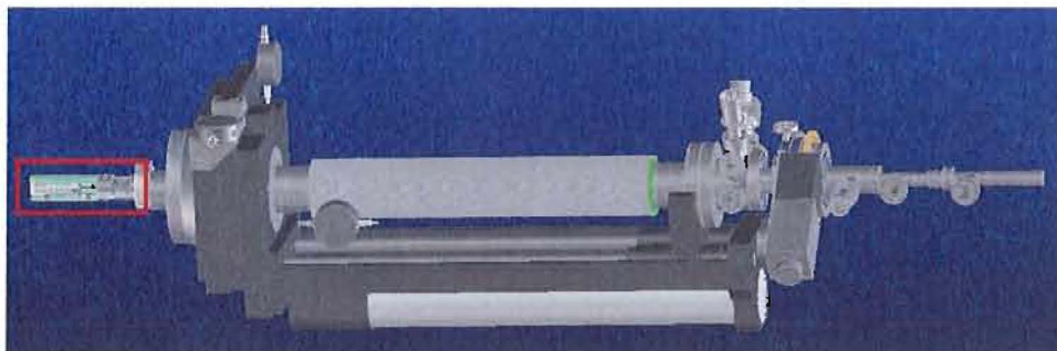
Fig. 6.7: Manipulator The sample manipulator is shown with the pinhole mechanism attached to the end. The large cylinder at the center of the manipulator is a 4.5 inch bellow needed when the sample is transferred into the center of the chamber. The cryostat is in the center of the cylinder and is connected to a liquid helium or nitrogen supply from the back end. The five feedthroughs near the back end are for bender and inchworm control, feedback for each, and a sample current readout.
