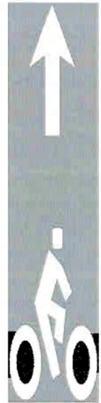
Bicycle lane pavement stencil and arrow
