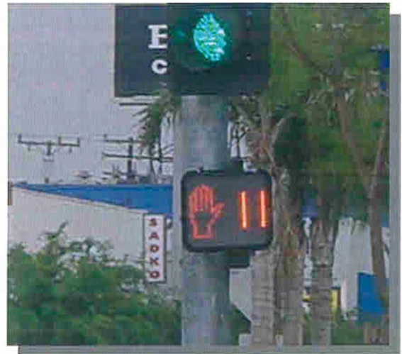
Pedestrian crossing countdown signal
