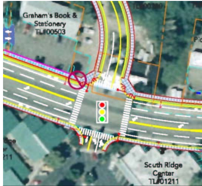
New Traffic Signal on Beaver Creek Road to the Younger Property and Southridge Center included as part of Short-Term Plan.
