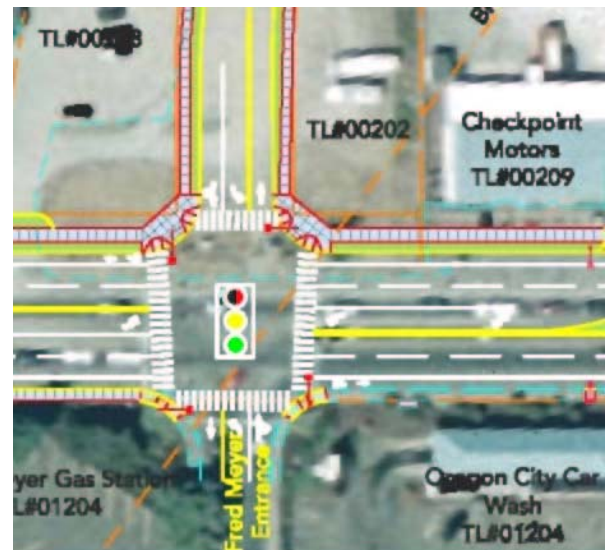
Signalized access to property #10
