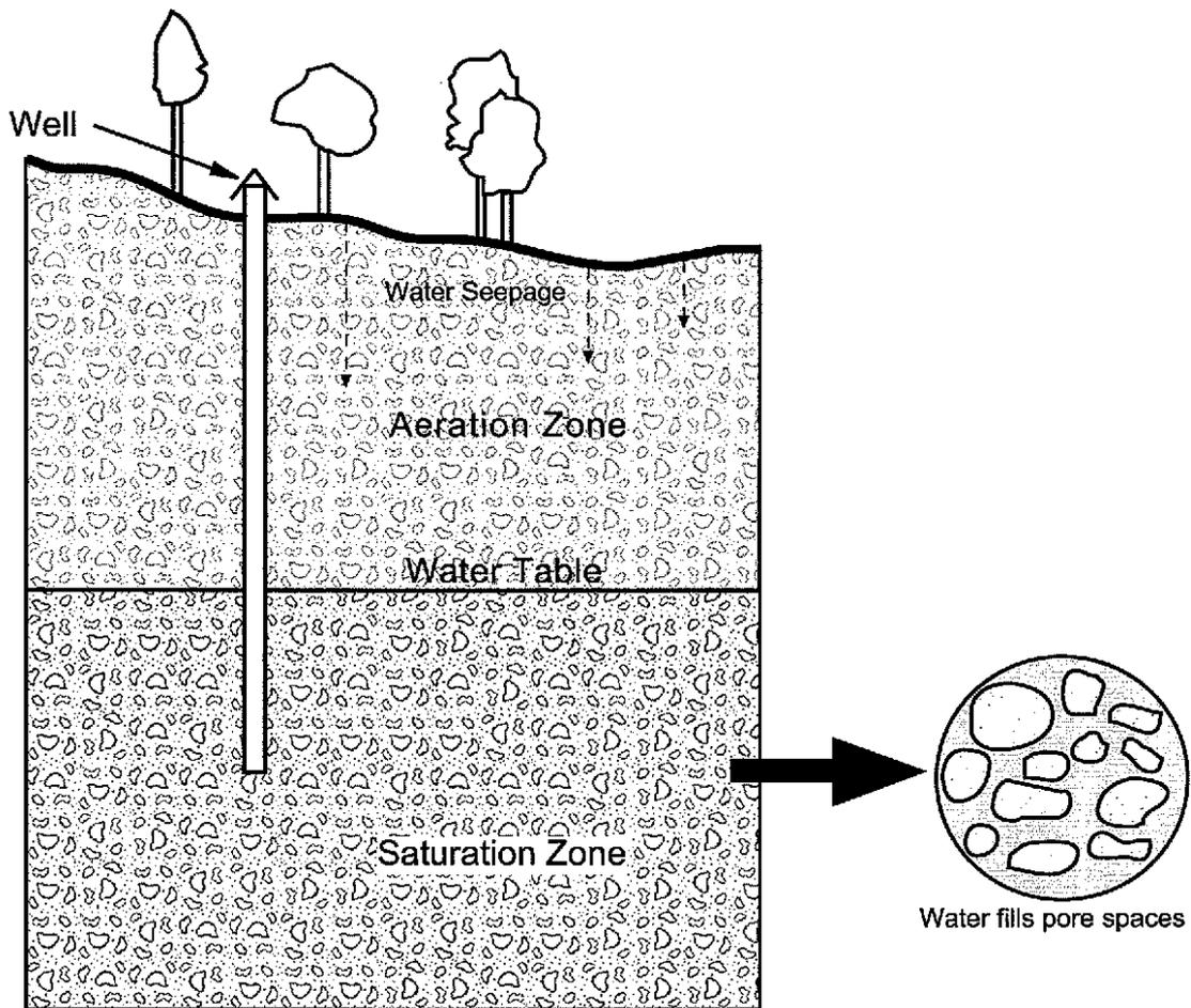
Groundwater occurs in the saturated zone. In this zone spaces between particles, the pores, are completely filled or saturated with water. Wells enter this zone and access the stored water. The zone of aeration typically has some water in the pores while the rest of the space is filled with air.
