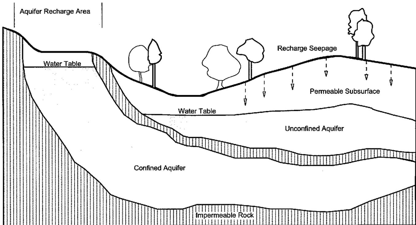
Seepage from the surface permeates through the subsurface and collects in an unconfined aquifer. An unconfined aquifer is more susceptible to contamination as water permeating through the subsurface, possibly carrying contaminants with it, enters the unconfined aquifer.
