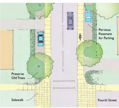
Figure 17: Enlarged Plan with On-Grade Sidewalks, No Bike Lanes and Casual Parking
