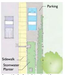
Figure 18: On-Grade Sidewalk and Stormwater Planter
