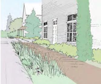
Figure 11: Proposed Stormwater Planter and Boardwalk at Historic
