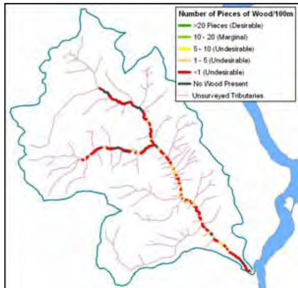
Figure 2-21: Large Wood in Tryon Creek. The number of pieces of wood per 100 meters of stream length. Scientists consider 20 or more pieces per 100 meters of stream length desirable. The vast majority of Tryon Creek has less than 1 piece of wood per 100 meters, significantly less than desired conditions. To view this map in color visit www.river.ci.portland.or.us .
