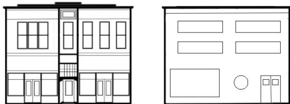
Figure 22: Varied, generally symmetrical window spacing at left, with asymmetrical openings at right. Overtly asymmetrical openings such as these are typically incompatible with traditional downtown architecture.
