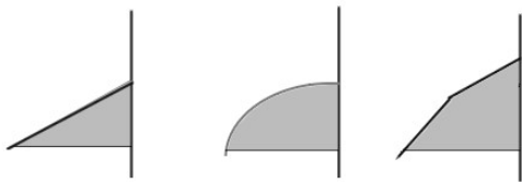
Figure 32: Awning Profiles, (Single Slope, Bubble and Multi-Slope)
