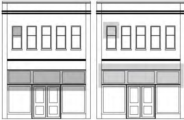
Figure 34: Awning Locations Within the Bay Outside the Bay
