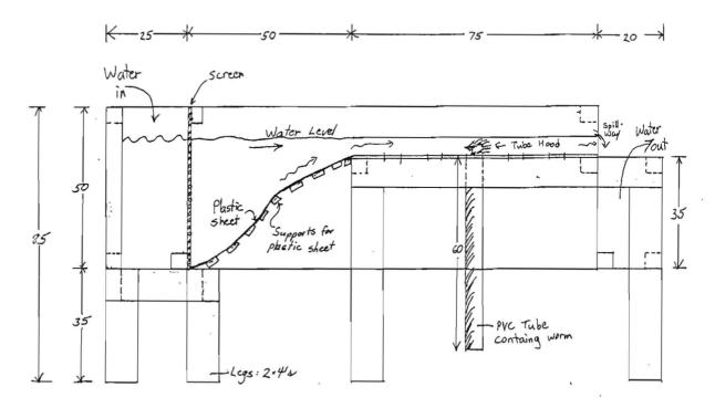
Side View - Shown with plywood sides removed. Plywood is 98"
