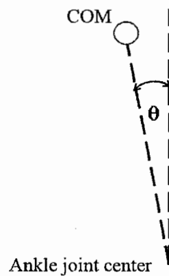
Figure 3.1. An illustration of the center of mass (COM)-ankle joint center inclination angle in the frontal plane
