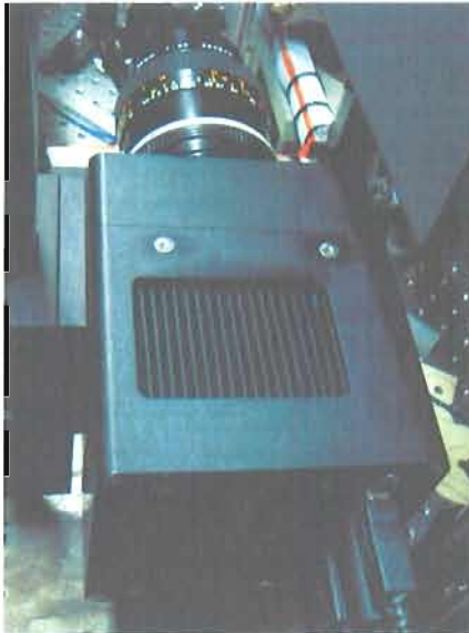
FIGURE 3.27: The MicroLine CCD camera equipped with a macro lens used to image atoms.
