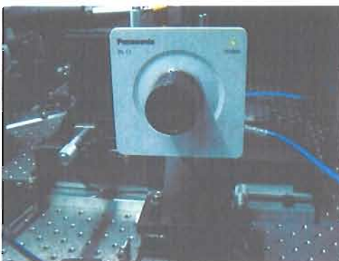
FIGURE 3.29: The Petcam works as an inexpensive beam profiler.
