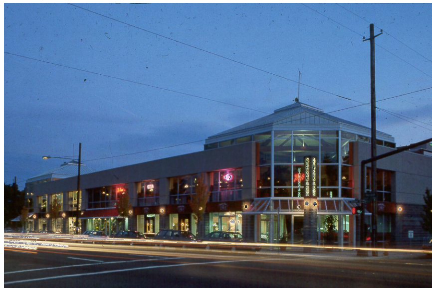
Architecture can create a sense of gateway by accenting building corners with enhanced facade lighting.
