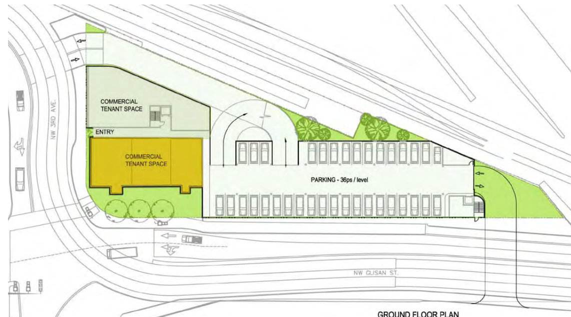
Ground and Typical Floor Plans indicating a renovated fire station, parking accessed from both the east and west, and either commercial or housing uses above
