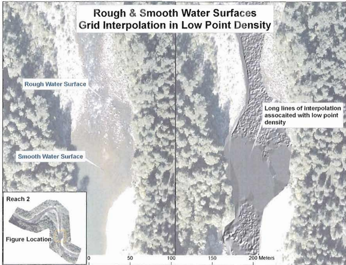
Figure 21. LiDAR Point Density versus Interpolation. Side by side image showing long lines of interpolation associated with smooth water surfaces (right image). Smooth water surfaces tend to have low LiDAR point density. The image on the right shows a hillshade of the LiDAR DEM. The DEM has been visualized using a 2 standard deviation stretch to highlight long lines of interpolation.
