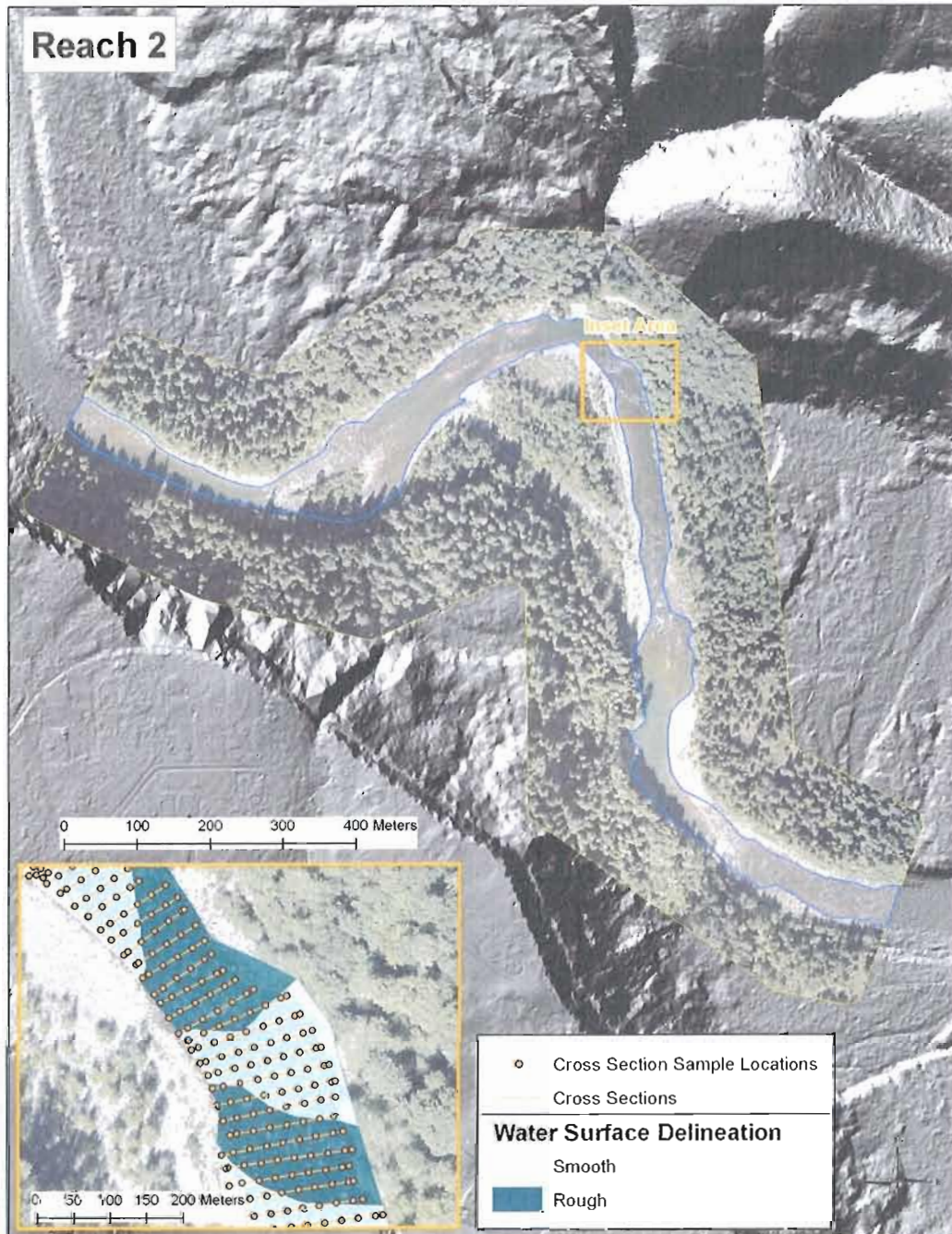
Figure 9. Reach 2 Site Area Map. Site map of Reach 2. Reach 2 contains 359 cross sections derived from LiDAR and 3,456 sample points. Inset map shows cross section sample locations derived from LiDAR and smooth/rough water surface delineations used in analysis.
