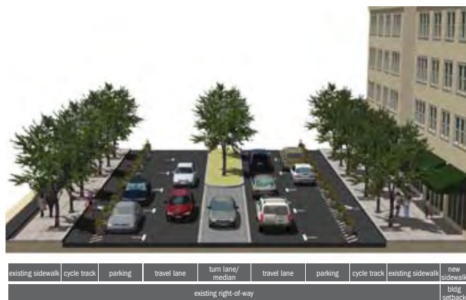
Capitol Highway design concepts The two design concepts above present a streetscape with a center median, wide sidewalks, pro-time parking lanes, and variations on a cycle track. Any future re-design of Capitol Highway would require significant study to assess traffic impacts and safety for all modes of transportation.
