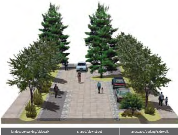
Dewitt Street extension concept One design consideration for the north-south segment is a curbless street that preserves existing large trees.
