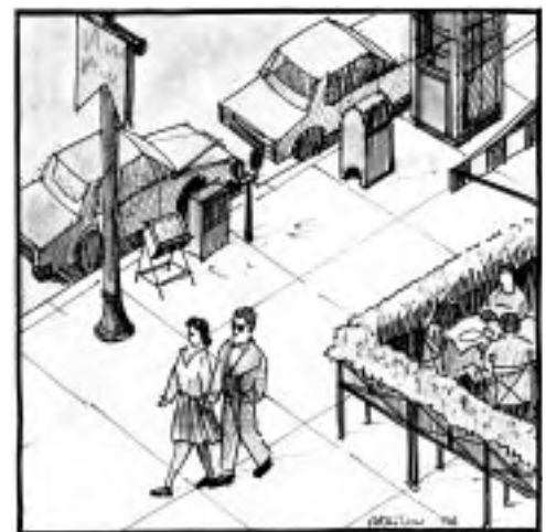
The Furnishings Zone buffers pedestrians from the roadway and is the place for elements such as street trees, poles, parking meters and street furniture.
