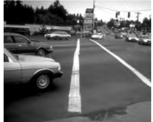
Very long crosswalks discourage pedestrian travel. Designers should avoid making crosswalks longer than 15 m (50'-0"). For wider streets, consider the use of median refuge islands.
