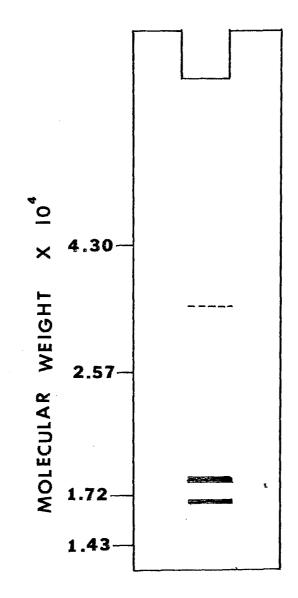
Figure 11. Sodium dodecyl sulfate slab gel electrophoresis of <u>Cucumaria miniata</u> hemoglobin. Gel consistancy 15%.
