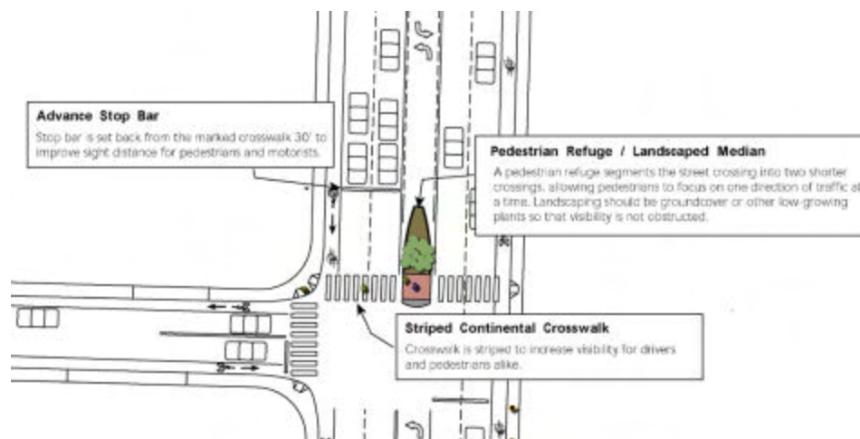
Figure 5-10. Type 1+ Crossing with Median
