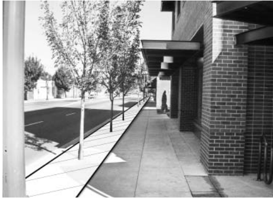
The furnishing zone (FZ), from the back of the curb to the sidewalk, allows for the installation of both horizontal and vertical pieces but these must integrate with other street furnishings including street trees.
