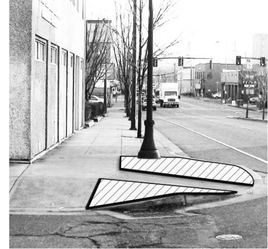
Installation in areas such as curb bulb-outs may be three dimensional but these occur only sporadically along the boulevard and objects can not disrupt traffic or pedestrian views at intersections.
