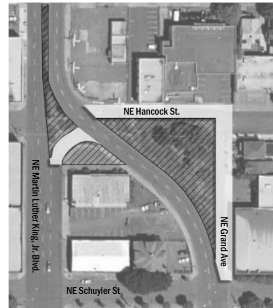
Areas highlighted in figure (bottom right) were proposed for the addition of specialty paving and sidewalk enhancements.
