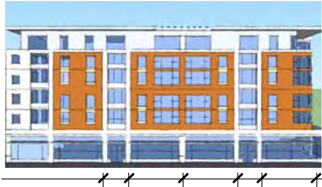
Fig. B.2.d.1 & 3 belt line above ground level and regular cadence of bays and storefronts framed by pilasters
